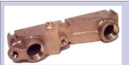
Raypak uses standard bronze headers for domestic hot water boilers. Failure to provide a non-ferrous waterway will result in oxidation and lead to costly heat exchanger replacement.
